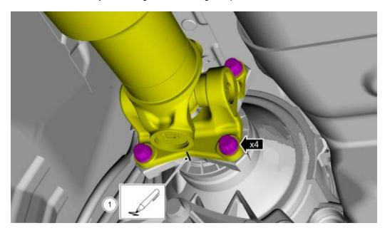
STEP 11: Remove the driveshaft center bearing bolts and remove the driveshaft. Clean and remove any remaining thread locking compound on the removed bolts.
