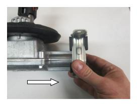
**STEP 16:** Remove anti rattle clip for the shifter lever if equipped.
