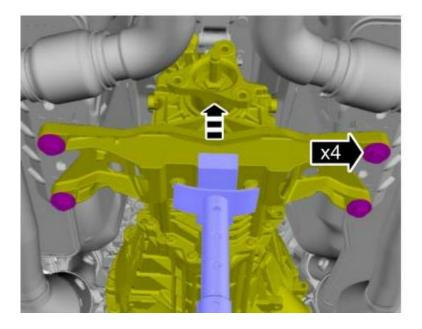
STEP 46: Install the driveshaft using the center bearing bolts with Blue thread locking compound. Torque: 35 lb.ft (48 Nm)
