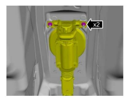
STEP 14: Remove the gearshift lever-to-transmission bolt (1). Remove the gearshift lever bolt (2). Remove the gearshift lever assembly from the transmission by pulling towards the rear of the vehicle.
