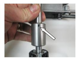
STEP 29: Slide the new shift lever into the housing, once again, verify the reverse lockout shoulder bolt hole is orientated towards the left side while seated in the driver's seat.
