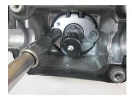
**STEP 31:** Align actuator arm bushings into the shifter housing and lower shifter pivot.
