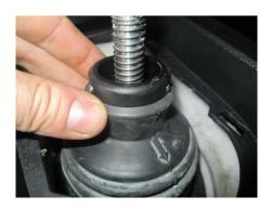
**STEP 38:** Install the anti rattle clip over the shifter lever until it rests on top of the roll pin if equipped.
