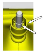
**STEP 53:** Evenly tighten the (3) 5/64" set screws in the reverse lockout against the ring on the gear shift handle boot.
