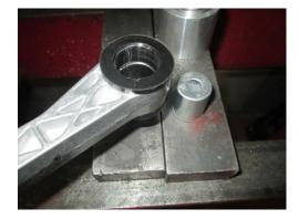
**STEP 40:** Remove both halves of the front bushing.
