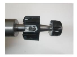
STEP 28: Verify the hole for the reverse lockout shoulder bolt is orientated towards the left side while seated in the driver's seat.
