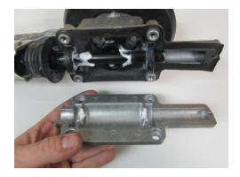
**STEP 22:** Remove the lower actuator arm by slowly lifting off of the lower shifter lever pivot. Do NOT remove the existing grease from assembly.
