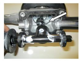
**STEP 23:** Remove (2) bolts from shift lever retaining plate. Remove plate.
