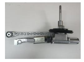
STEP 34: Apply provided grease to shift lever and install the provided reverse lockout sleeve over the new shift handle assembly and align slot to the shoulder bolt hole. Install the shoulder bolt with Red thread locking compound. Torque: 16 lb.in (1.8 Nm)
