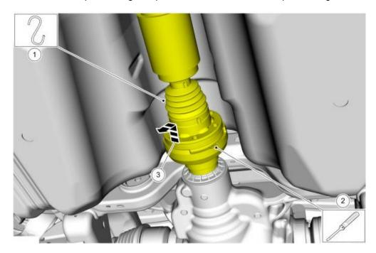
STEP 10A: If equipped with 3 bolt flange (If equipped with 4 bolt flange proceed to step 10B): Mark the driveshaft flex coupling to the transmission flange. Remove the driveshaft to transmission flange bolts. Position and support the driveshaft aside. Clean and remove any remaining thread locking compound on the removed bolts.
