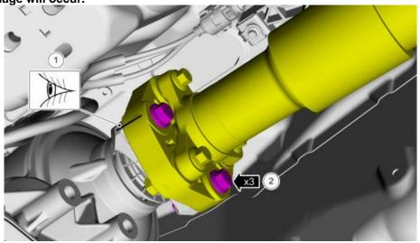
STEP 49: If equipped with 4 bolt flange: Align the index-mark on driveshaft flex coupling to the transmission flange. Install the driveshaft flex coupling to transmission flange bolts with Red thread locking compound. Torque: 80 lb.ft (109 Nm)
