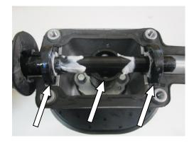
STEP 32: Install the provided housing gasket onto the shifter assembly. Slide the lower housing cover into place. Install (4) bolts with Blue thread locking compound. Torque: 75 lb.in (8.5 Nm)
