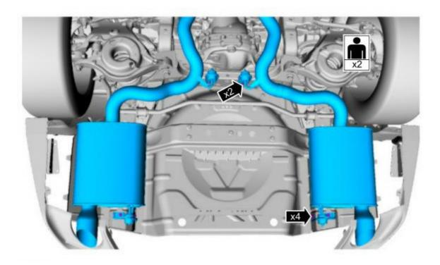
STEP 51: Slide the clamps from the tailpipes over the RH and LH catalytic converters. Tighten clamps. Torque: 35 lb.ft (48 Nm)
